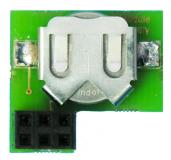
The module can now be fitted onto GPIO pins 1-6 of the Raspberry Pi.
